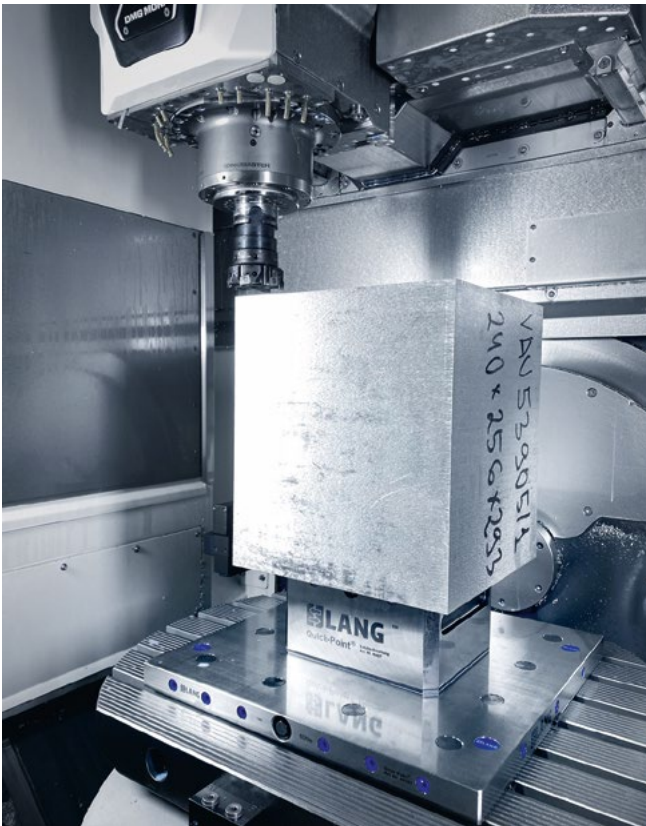
Not only highly precise, but also highly resilient. Four clamping studs are screwed directly into the workpiece, which weighs about 50 kg.
