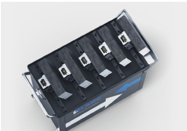
Automation trolley with standard alignment. Here 5 parts, each measuring 410 × 205 × 90 mm.
